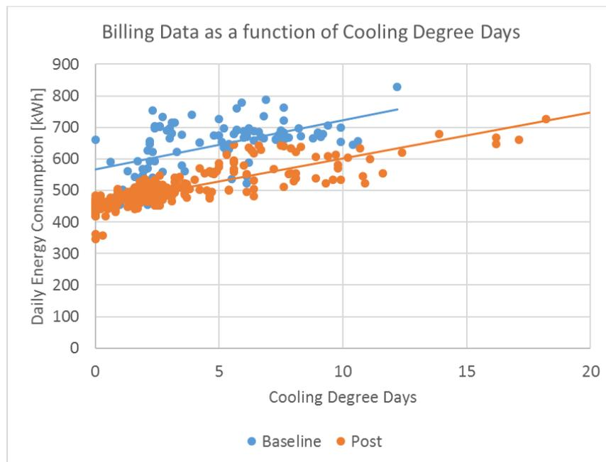
A multi-variable linear regression to CDD and HDD for daily billed energy consumption was established for the baseline and post-measure periods. This regression analysis resulted in an estimated annual total site baseline energy consumption of 219,877 kWh and 13.2% energy savings of 28,918 kWh.
