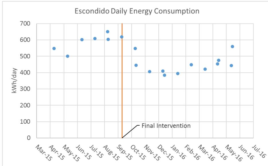
In order to estimate annual savings using the utility metering data, a regression of daily energy consumption to daily heating and cooling degree days was established. There is a clear reduction in energy as seen in Figure 7. Note that the majority of system performance improvement is seen at part load performance days whereas peak cooling days see roughly the same energy consumption. No dependence on weekday was observed.
