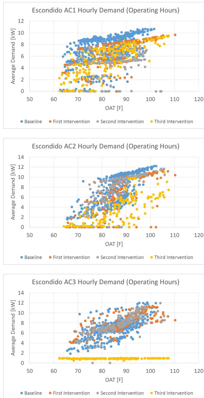
Figure 23 shows the hourly-averaged measured demand for each unit across each measurement period. Note that RTU1 was a unit that had to be replaced prior to the baseline. As a result, the first two stages (deep maintenance and air balancing) appear to have had little to no effect on the performance, as you would expect on a new unit.
