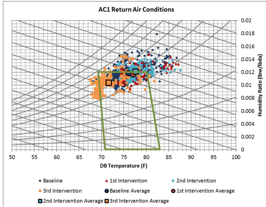
FIGURE 17 – RETURN AIR CONDITIONS FOR EACH MONITORING PERIOD (ESCONDIDO – RTU2)
