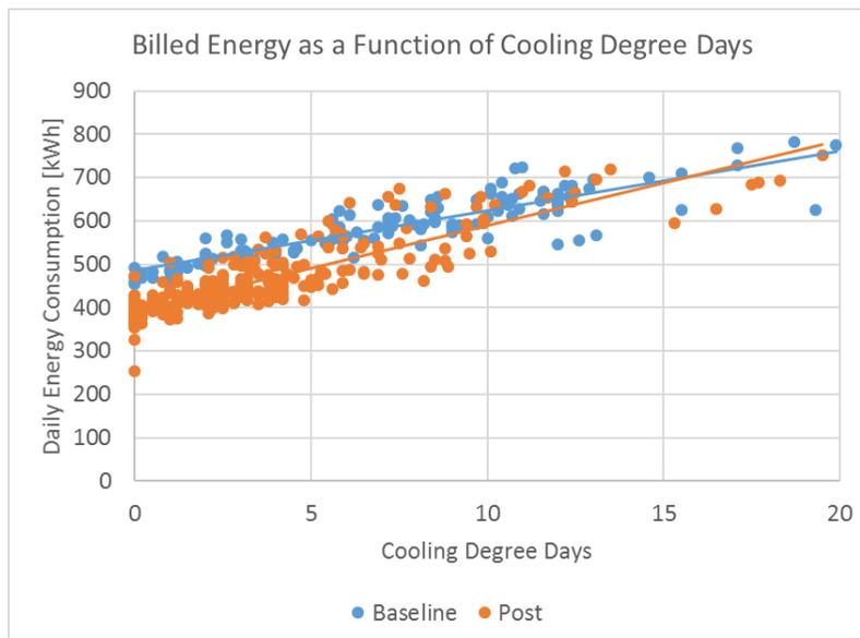
A multi-variable linear regression to CDD and HDD for daily billed energy consumption was established for the baseline and post-measure periods.
