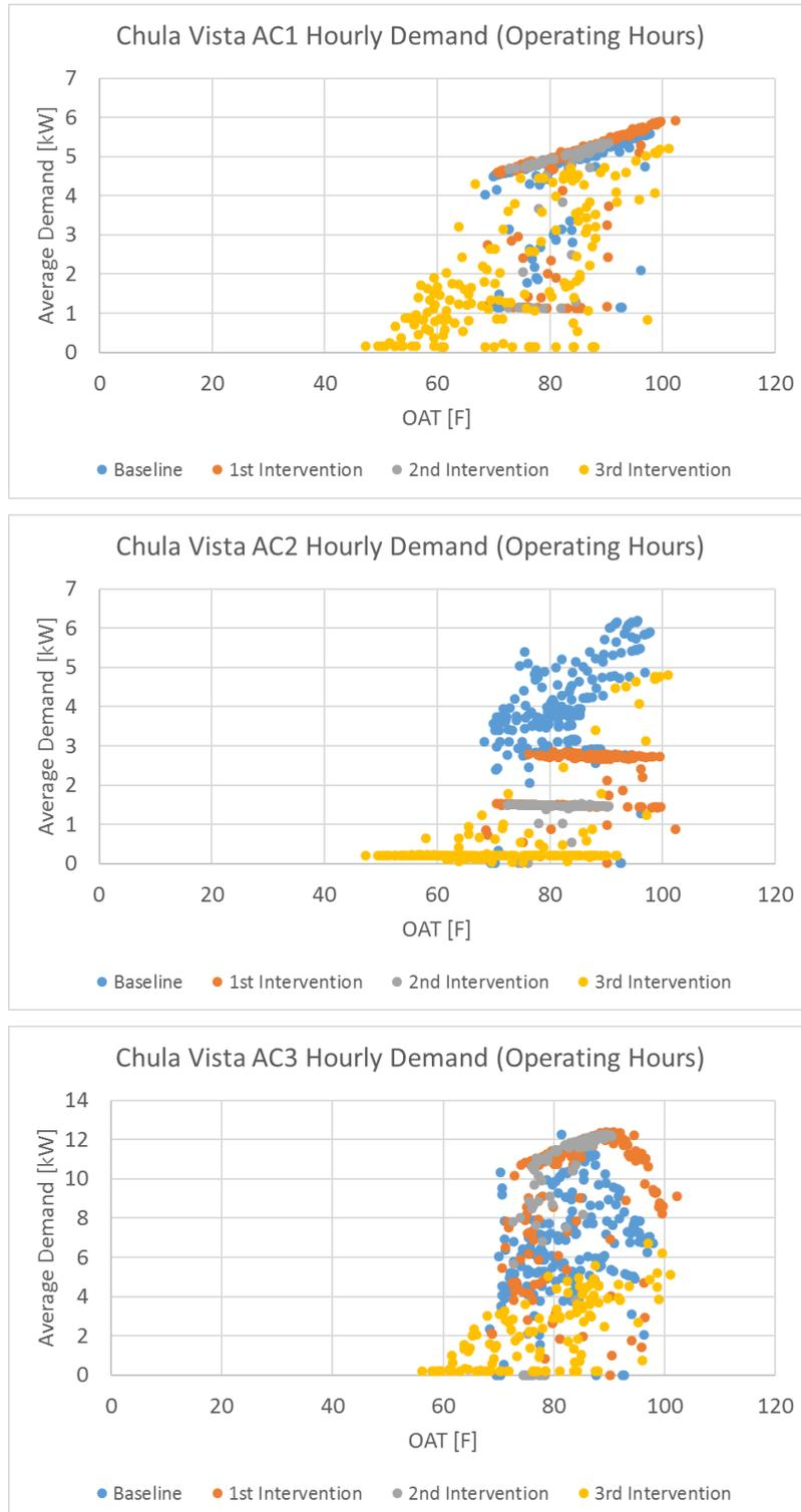
Power and operating condition variables were recorded in order to develop an annualized model for each RTU for the baseline and each stage of the optimization. The only regression that provided meaningful results was a simple regression of daily energy use to cooling degree days. Hourly data had too much variance to establish useful regressions on an hourly basis to monitored variables such as outside air conditions, operating hours, and humidity.
