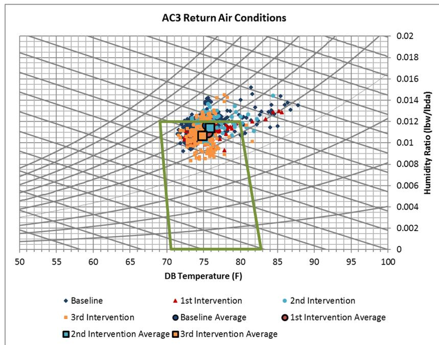
The following figures plot the hourly and average psychrometric indoor air conditions for each RTU and monitoring period in Chula Vista during operating hours.
