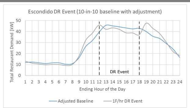
FIGURE 8 – DR DEMAND CURVES FOR THE 1F/HR TEST (ESCONDIDO)
