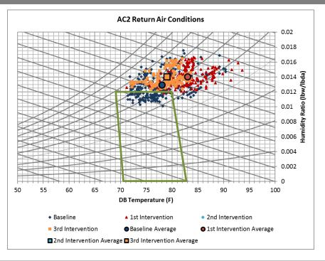
FIGURE 20 - RETURN AIR CONDITIONS FOR EACH MONITORING PERIOD (CHULA VISTA - RTU2)
