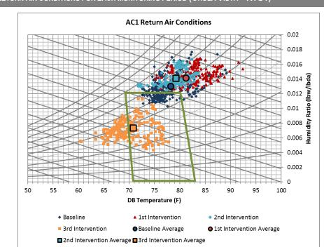
FIGURE 19 – RETURN AIR CONDITIONS FOR EACH MONITORING PERIOD (CHULA VISTA – RTU1)
