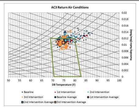
FIGURE 18 – RETURN AIR CONDITIONS FOR EACH MONITORING PERIOD (ESCONDIDO – RTU3)
