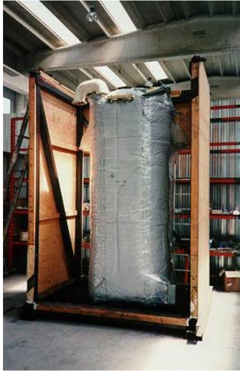
Figure 3 - 200 kW PAFC Stack Assembly (Source: Ansaldo CLC)
