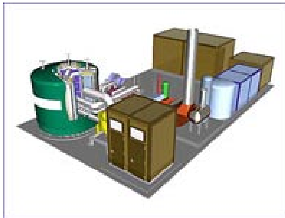
Figure 14 - FCE 1 MW MCFC Power Plant (Source: Fuel Cell Energy, Corp.)
