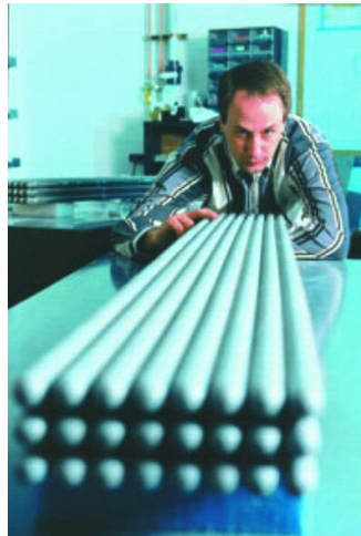
Figure 6 - Siemens Westinghouse SOFC Stack Tubes (Source: Siemens Westinghouse)
