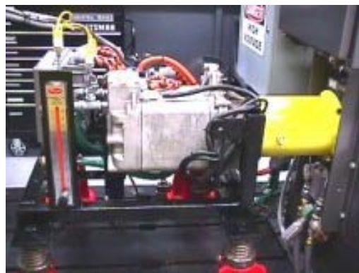
Figure 23 - Siemens Electric Motor Drive Under Testing (Source: US DOE Argonne National Laboratory)
