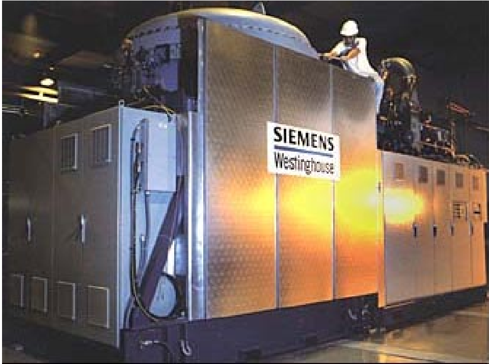
Figure 16 – Hybrid SOFC 300 kW Power Plant (Source: Siemens Westinghouse)
